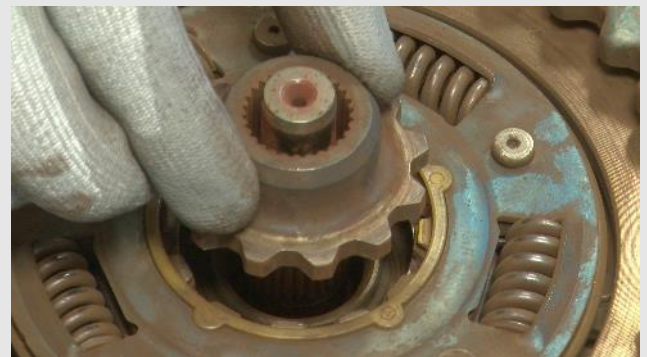
STEP 4 - Remove manually the top hub of DDC package
