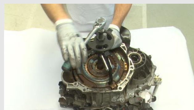
STEP 7 - Screw it using a wrench (19) until DDC bearing is completely removed from the primary shaft.
