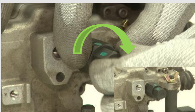
STEP 5 - Rotate the adjuster to get the correct length. 4 revolution will be 1mm of cylinder displacement. Rotations: Lever 1 : 72 \text{ mm} - 59 \text{ mm} = 13 \text{ mm} * 4 = 52 \text{ tool turns} Lever 2 : 72 \text{ mm} - 32 \text{ mm} = 40 \text{ mm} * 4 = 160 \text{ tool turns}
