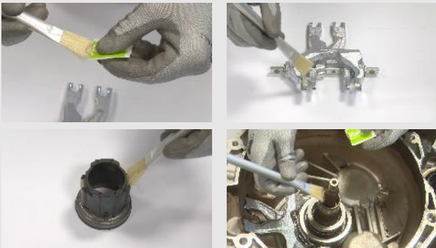
STEP 5 – Add the quantity of grease necessary in forks, bearings and spline shaft
