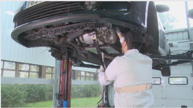
STEP 1 - Remove the gearbox using a hydraulic lift table.
