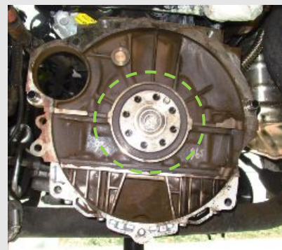
STEP 2 - Inspect the crankshaft seal, if any presence of leak or damage . Repair it if needed before fit the new flywheel
