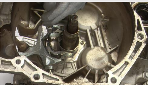
STEP 7 - Tighten 3 screws (M6) to fix new forks to gearbox housing. Mount release bearing. Use Allen wrench 5- Tightening torque 15Nm: only fits in one position
