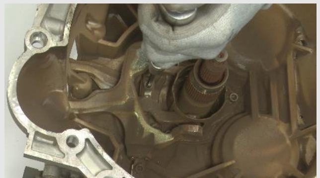
STEP 2 - Remove both release bearings and 3 screws that fix the guide tube to the gearbox. Use Allen wrench 5
