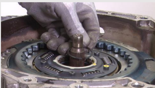
STEP 7 - Mount the inner snap ring a pliers
