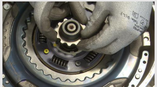
STEP 8 - Insert manually the hub on the DDC package
