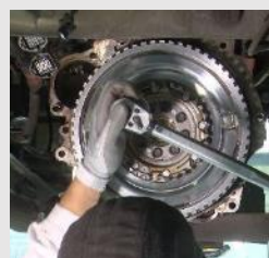
STEP 4 Apply progressive torque following a star sequence. Tightening torque 110Nm
