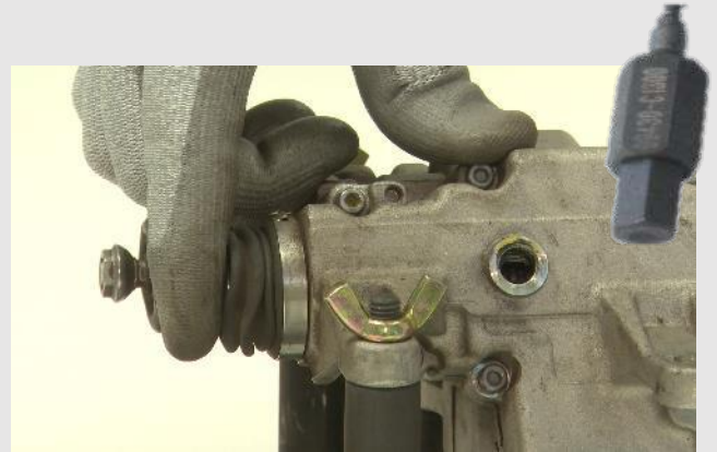
STEP 4 - Push completely until stop end the cylinder and insert the actuator adjuster (DDCT-04) on the hole. The final length of both cylinders must be 72mm.
