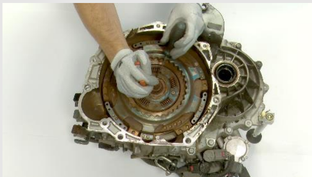
STEP 3 - Remove the snap ring from the upper hub of DDC package with the snap ring pliers
