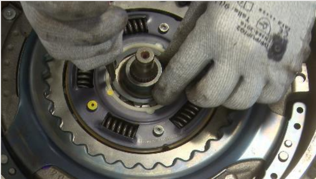
STEP 9 – Insert the outer snap ring with a pliers
