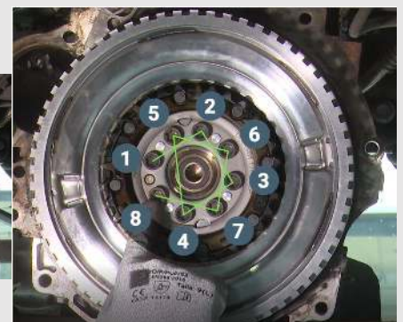
STEP 4 Apply progressive torque following a star sequence. Tightening torque 110Nm
