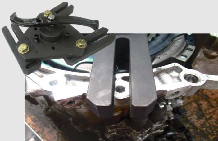
STEP 5 - Fix the DDC installer tool (DDCT-01) on the gearbox on 3 holes with original gearbox screws
