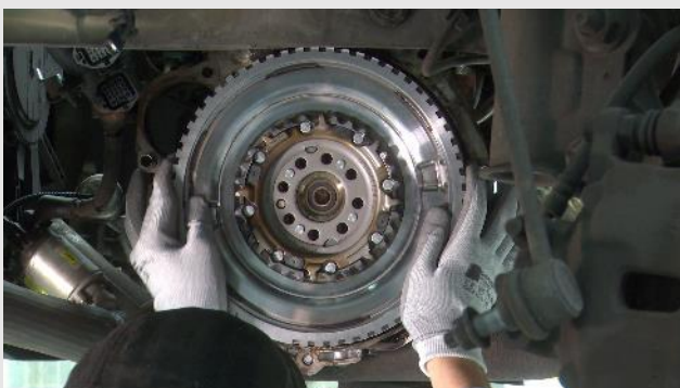
STEP 3 - Position the new flywheel tightening manually the bolts M10x1
