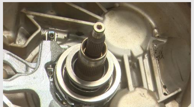
STEP 8 - Check if the release bearings can slide correctly by acting manually on the dual fork
